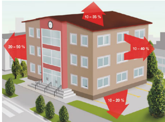
Fig. 57.1 Places from where the heat escapes. Source http://www.termoviznemeranie.com/
